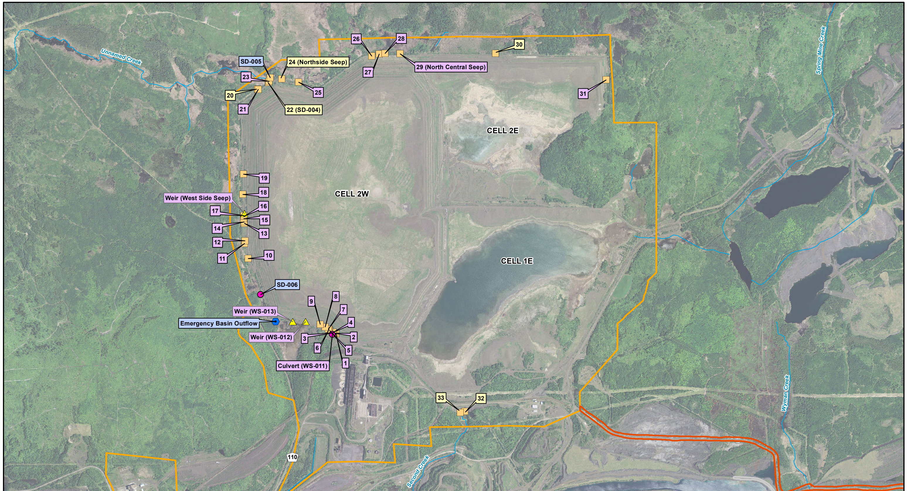
Figure 4.2-11 Seeps and Associated Flow Structures at Existing LTVSMC Tailings Basin NorthMet Mining Project and Land Exchange SDEIS Minnesota
